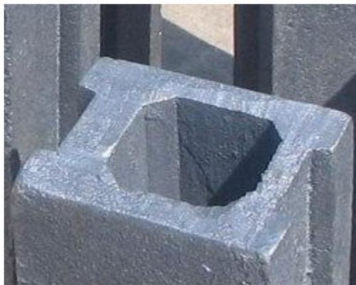
**Raised Mold Defect**
