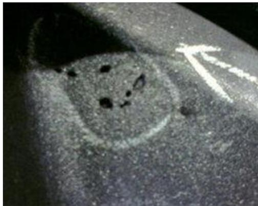
**Shrinkage Cavity Defect**
