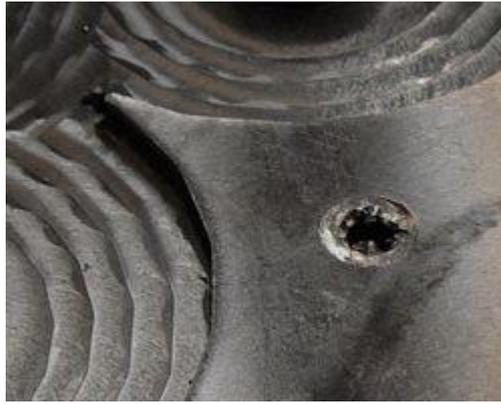
**Uneven Hardness Defect**
